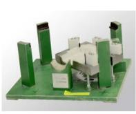
Fig. 7. Fixture for operation II
